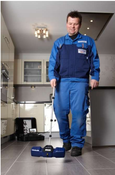
Fig. 7: Localizing the camera head underground
